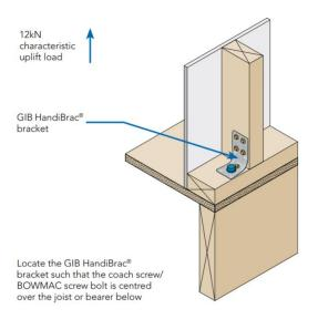
Figure 2: HandiBrac on external joist <u>https://www.gib.co.nz/assets/Uploads/LiteratureFile/PRODU</u> <u>CTS/GIB-HandiBrac-Brochure.pdf</u>
