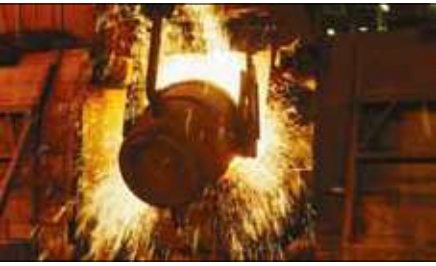
Above: Molten Iron being charged into the steelmaking vessel.
