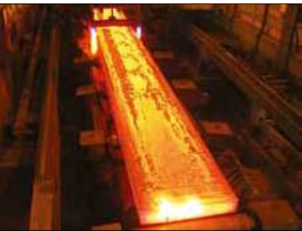
Above: Steel Slab emerging from the casting machine.
