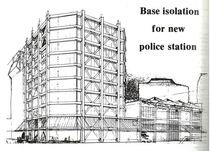
A base isolated cross-braced frame was selected by the designers of a new Wellington Central Police Station to ensure the high seismic performance required for an essential facility. The 10 storey tower block with a four storey car parking building alongside was designed by the Ministry of Works and Development and construction should begin early next year.
