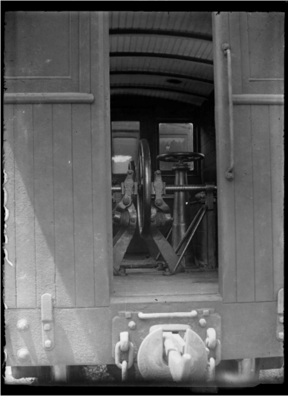
Figure 8: Interior of a Fell van, showing the hand and central rail grip brakes. Photographer: Albert Percy Godber. Alexander Turnbull Library. Ref: APG-0049-1/2-G. /records/22834928
