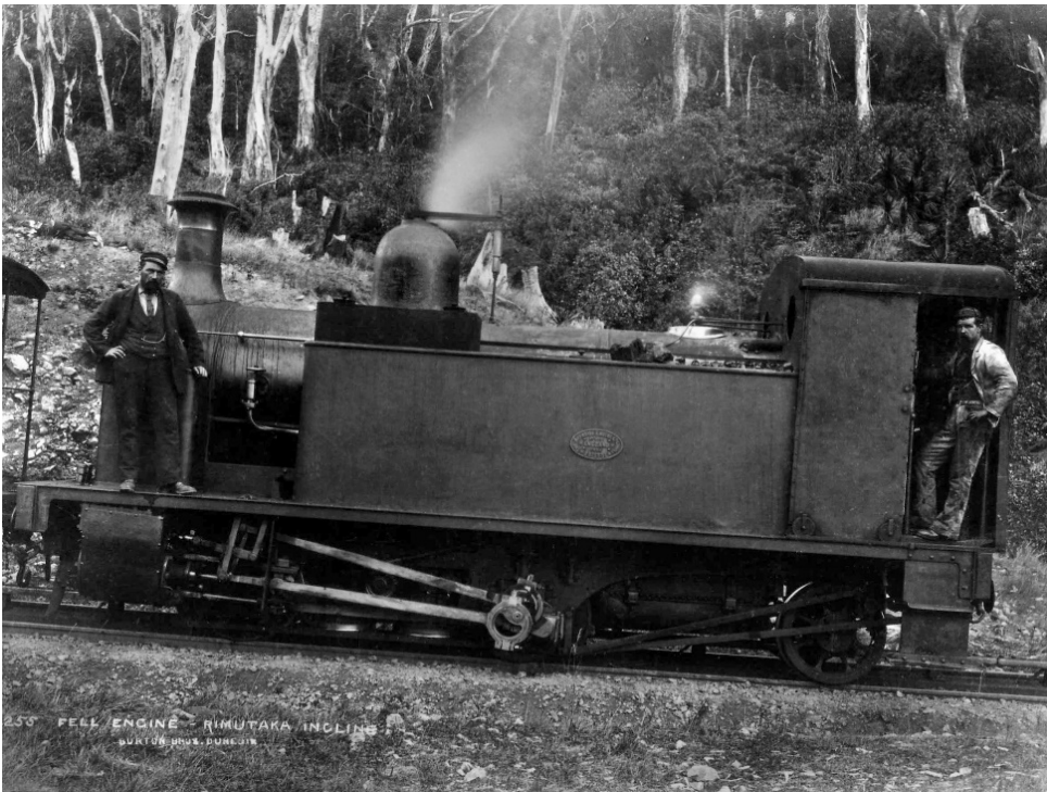
Figure 5: Fell engine at the Incline, ca 1890. Note the raised centre rail. Burton Brothers. Alexander Turnbull Library. Ref: PAColl-7581-31 / records/22877321
