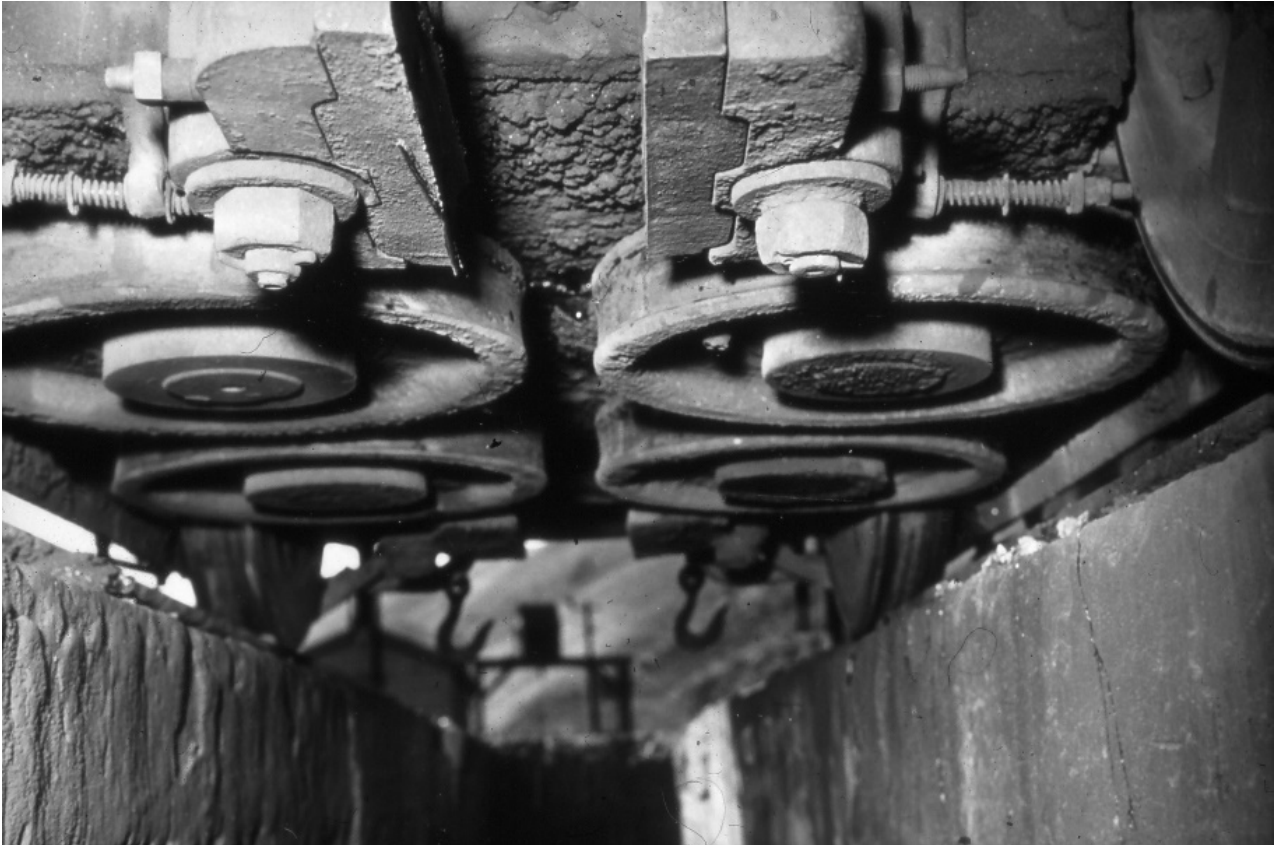
Figure 7: Underside of a Fell van, showing the horizontally aligned grip wheels. New Zealand Rail (NZR) Publicity Department Collection, negative number: B6327. Archives New Zealand.
