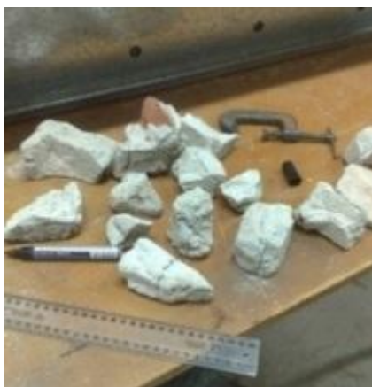
(a) Example of typical extracted mortar samples
