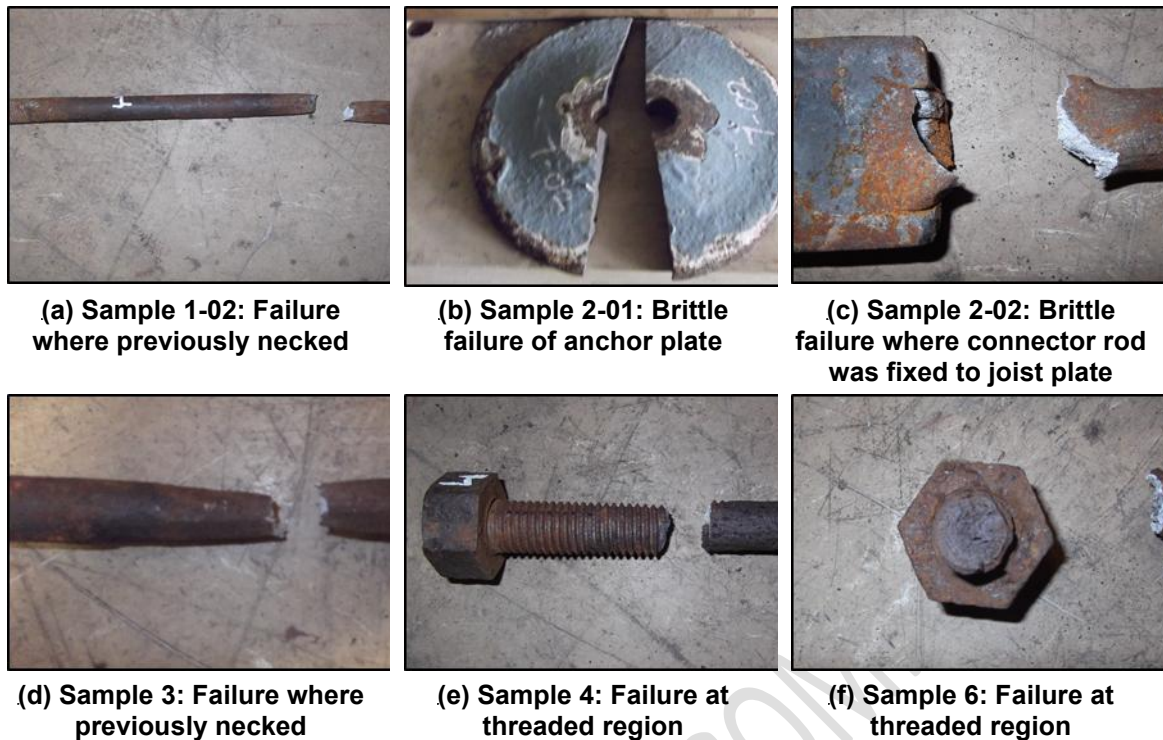
Figure C8.44: Observed failure modes from tensile test series (Campbell et al., 2012)
