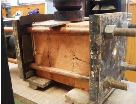
(a) Laboratory shear triplet test
