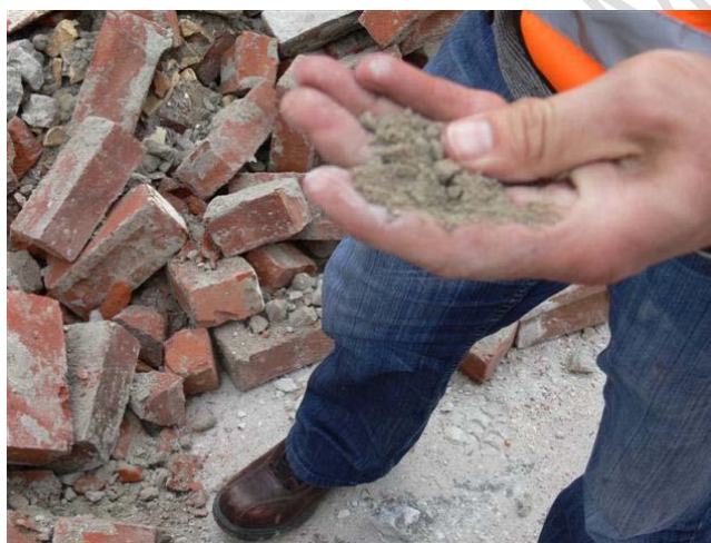
Figure C8.16: Soft mortar. Note the delaminated mortar from bricks in the background (Ingham and Griffith, 2011)
