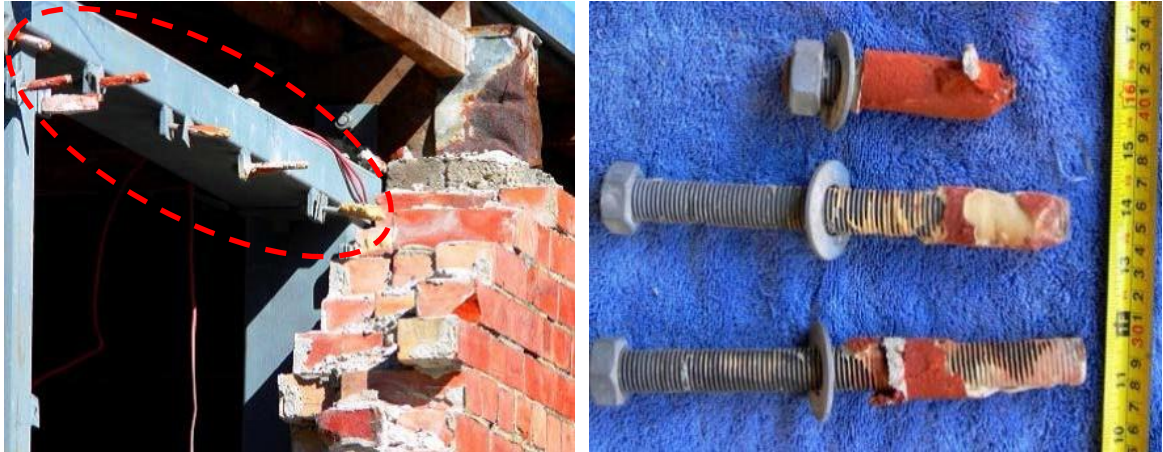
Figure C8.45: Failed adhesive brick anchors (Dizhur et al., 2013)
