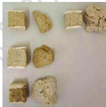
(b) Example of typical mortar sample preparations
