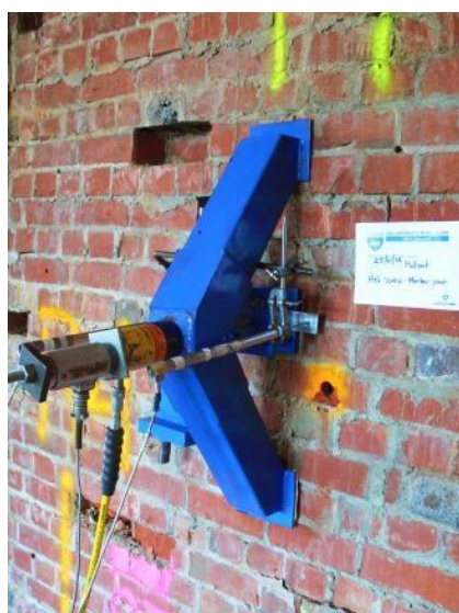
(a) Typical anchor pull test set-up
