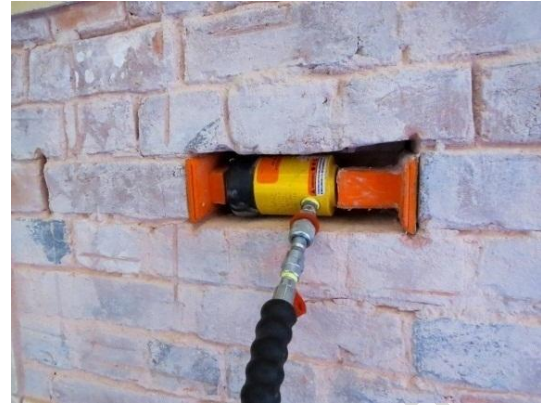
(b) In situ shear test without flat jacks (EQ STRUC Ltd)
