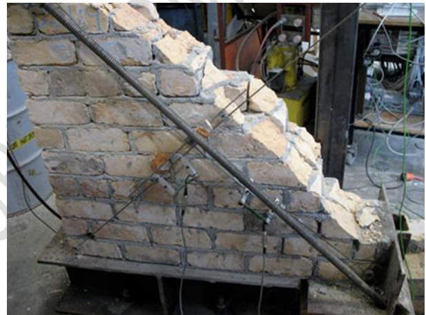
(b) Diagonal tension cracks to brick masonry. Note splitting of bricks, indicative of mortar stronger than bricks (Russell, 2010)
