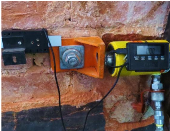
(a) Typical anchor shear tests set-up (push cycle)
