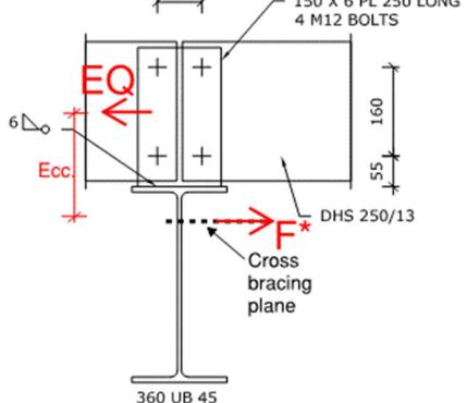
Load path just to get from DHS Strut to tension bracing
