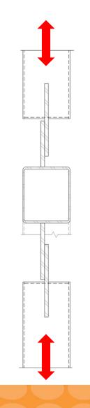
This connection cannot transfer the loads required No redundancy in bracing – this is the only structural element to transfer first floor/roof forces to ground floor
