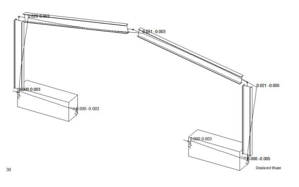
All the details shown provide 'fixity', but with different levels of modelling our displacements went from height/307 to height/190
