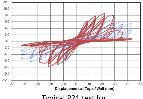
Typical P21 test for plasterboard lined wall
