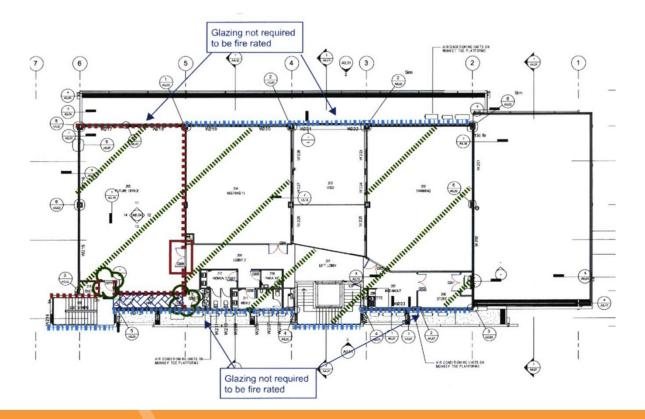
Fire Engineer required that the side walls on both the ground floor and mezzanine required post-fire stability
