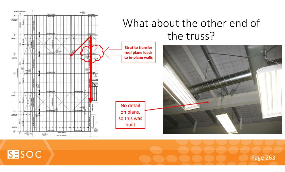
Builder has 'noded' the bracing with the roof purlins, not with the strut that is meant to transfer the loads!
