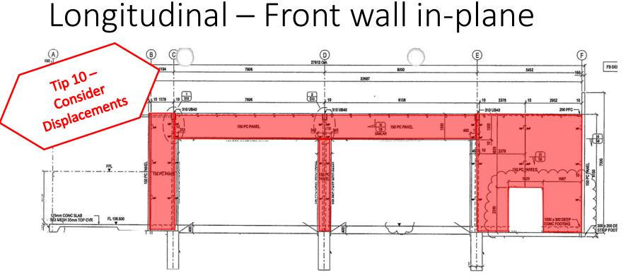
• Relative stiffness means the end panel will try and brace seismic loads
