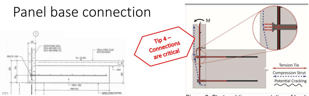
Proprietary insert, reliance on concrete in tension in cracked zone
