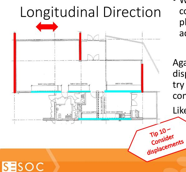
• We have out-of-plane precast concrete panels (red), and inplane BL1-H bracing walls (blue) acting in the same direction
