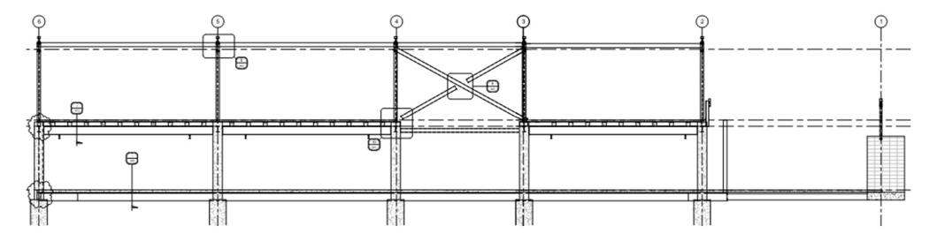
• Tension/compression brace in one bay to brace entire first floor roof and end walls out-of-plane
