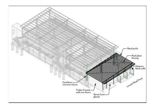
Formed with DHS purlins supported on a combination of cantilever masonry block walls, structural steel and timber framing
