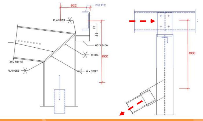
Load path just to get from Strut into angled wall strut
