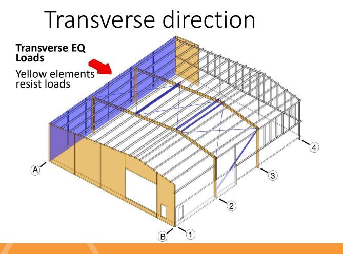
Seismic loads resisted by the steel portal frames and the inplane precast concrete panel end walls (shown yellow)
