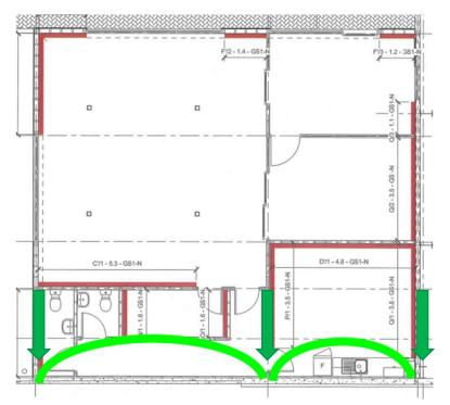
In theory the wall could have been propped by some structure at ceiling level
