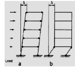
Comparison of Energy Dissipating Mechanism with and without Strong Column - Weak Beam Concept
