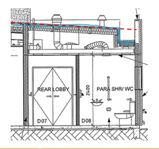
But roof plane is interrupted by the box-gutter – bracing cannot be installed
