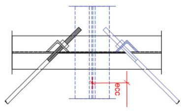
Connection detail – Roof Plane bracing to strut
