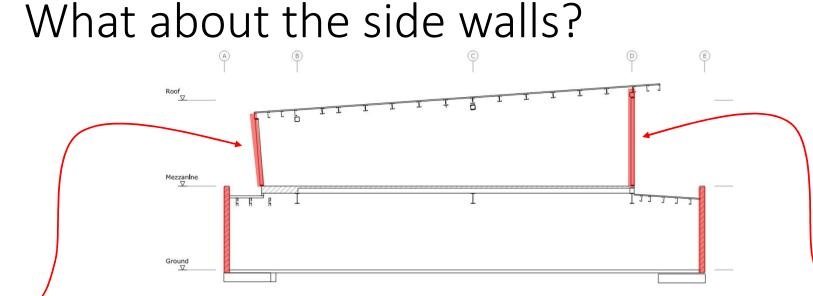
As talked about earlier – there was no engineered load path to support this wall out-of-plane
