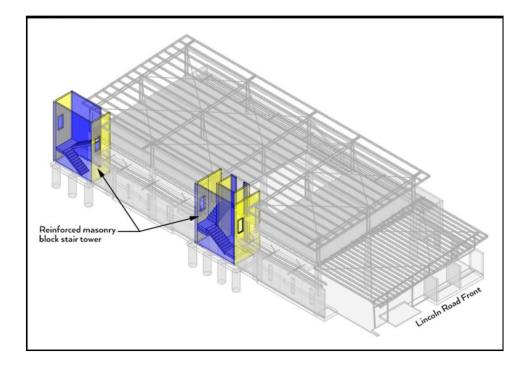
200 series reinforced masonry block stair towers
