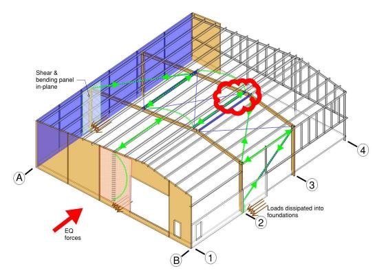
Joint between the purlins and the tension bracing
