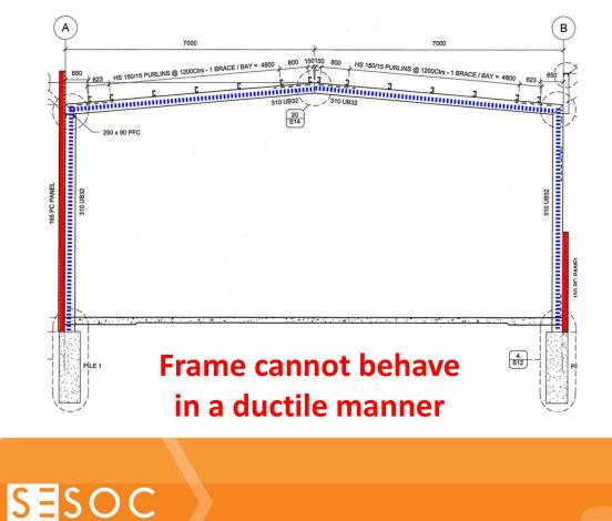
Foundations not designed to ensure yielding, ie not designed or checked for the overstrength capacity of the frame
