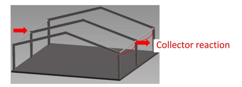
Reaction from the collector model was then applied to the portal frames
