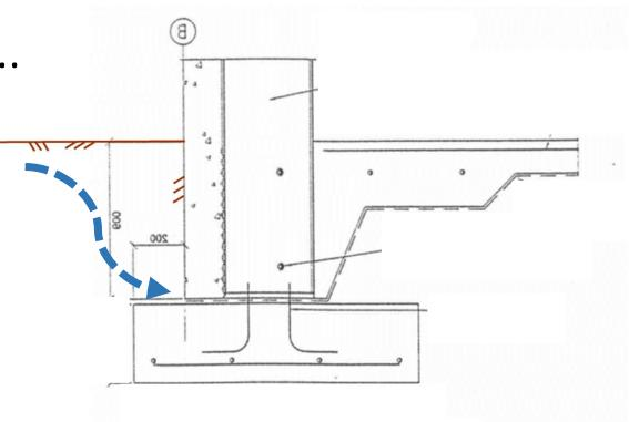
Implications – potentially unprotected structural steel susceptible to rusting
