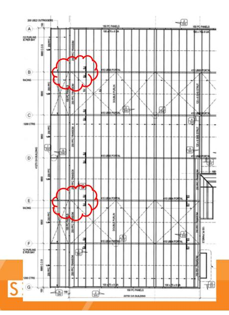
Roof plane bracing is meant to node here – transfer roof truss loads to the wall line in -plane
