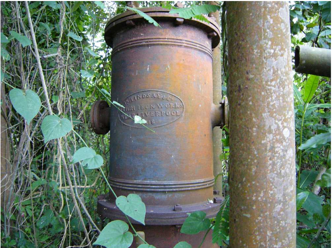
The international dimension. Cylinder of the beam engine of the Haiti sugar cane crushing mill, built by Lindsay & Co near Liverpool, 1818.
