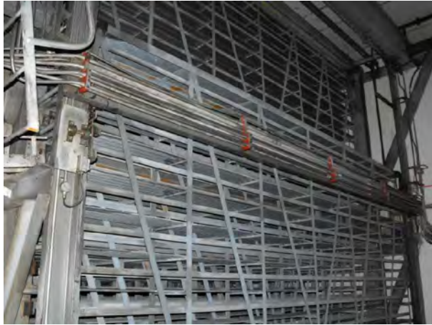
Figure 5: Load-in and load-out area of a continuous carton freezer – cartons are placed on the racks and transported along the freezer (with air cross-flow) to return on the upper level.
