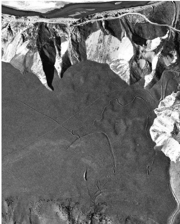
Figure 5. Medium format vertical of Muddy Terrace, dams at centre and bottom (total volume 5,200m 3 ), sluice faces and the Shotover River at top.
