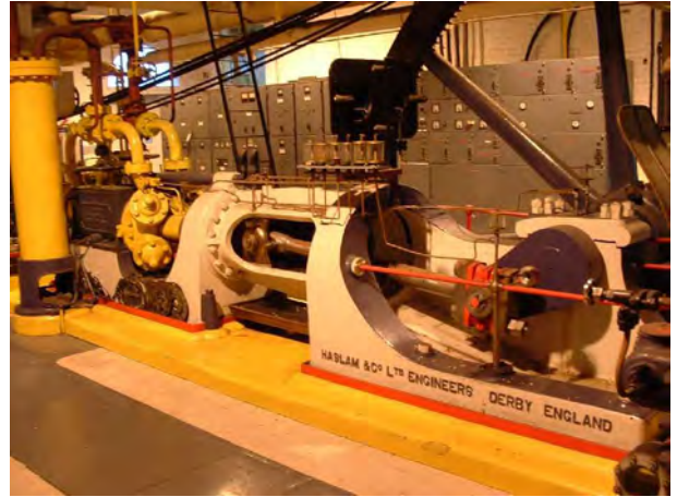
Figure 6: A horizontal open compressor with flywheel.
