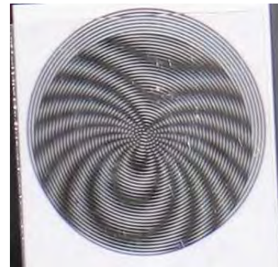
Figure 5 Moire telltale showing displacement
