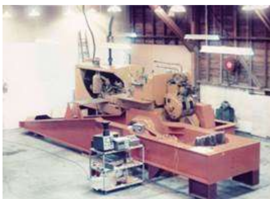
Figure 9: Masher when first built in 1974 for the twisting beam energy absorbers used in the South Rangitikei Viaduct, and being refitted in 1976 to develop the lead-rubber bearings. Sam Vanicek helps Cam (white shirt) to guide part of the test rig into place.
