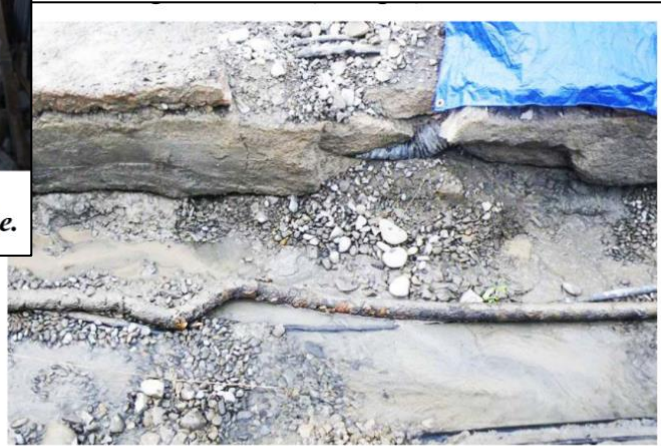
Figure 6: Earthquake damaged 11 kV steel and lead armoured cable, and above embedded in fractured concrete, a damaged 66 kV oil-filled cable.
